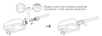
**2** The controller is connected Rope lights at the other end
